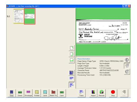
**5** Place an envelope onto the conveyor. The system will recognize the document as an envelope. In this example, an envelope is set up as the transaction boundary and ends the current transaction.
