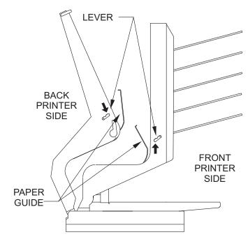
FIGURE 24: Printer release levers
