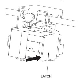
FIGURE 26: Cartridge lock down latch
