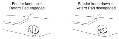
FIGURE 31: Feeder knob position
