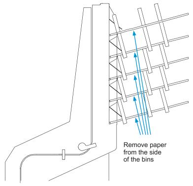
FIGURE 22: Clearing the output bins
