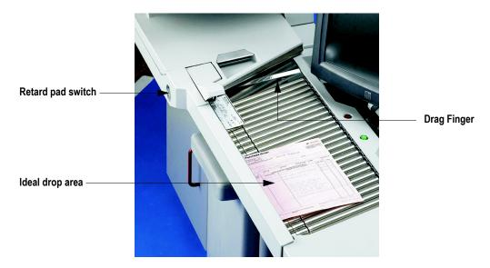
Since the feeder pulls from the top of the stack, the lead sheet in the stack must be the first to reach the feeder. If the bottom piece reaches the feeder first, a paper misfeed is likely to occur. There are techniques for learning to drop packets of paper consistently and effectively. The documents do not have to be perfectly aligned as long as the lead sheet is the top sheet. Review these techniques with your AS3600 Administrator or your OPEX Technician or Sales Engineer.
