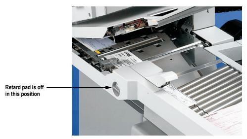
FIGURE 10: Adjust the retard pad switch
