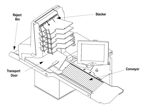
FIGURE 28: Conveyor and Stacker Assembly
