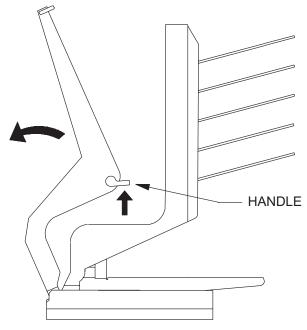
FIGURE 21: Opening the stacker transport cover
