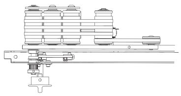
FIGURE 30: Feed Belt Assembly
