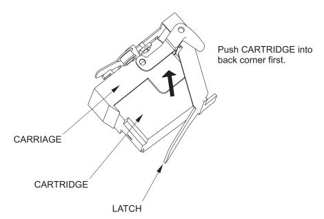
FIGURE 27: Installing the printer cartridge
