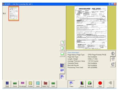
**4** Place the next document you want to scan onto the conveyor. In this example, the document is a check. The system recognizes the check by the presence of a MICR line at the bottom.
