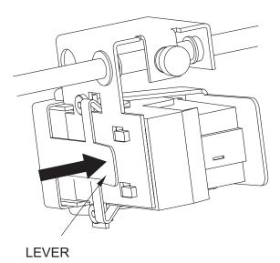
FIGURE 25: Cartridge release lever
