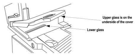
FIGURE 33: Cleaning the Contact Image Sensor glass surfaces
